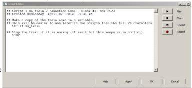
We then repeated this procedure for the other three trains waiting to be loaded. To do this we needed to change the reference in the SET command from T1 to read T2, T3 and T4 in each of the other scripts.
