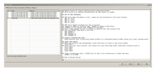
Once again we saved our file before moving on to Step Five. If we had moved any trains we would have needed to click the Rewind Button before saving. The next time we opened our file this Master Script executed automatically to set the variables, display the introductory note and start all four of the train scripts running.
